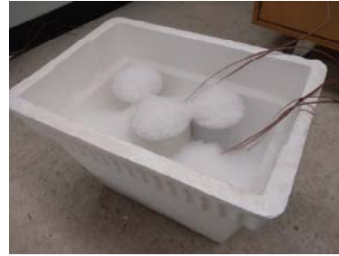
Figure 2: Dry ice environmental chamber
