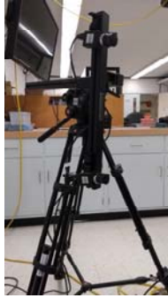
Figure 5: 3D DIC camera setup
