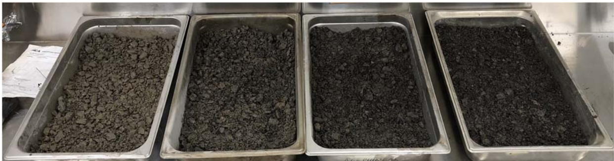
Figure 2: Samples Left to Right (Granular A - RAS) 100-0, 90-10, 80-20, 70-30
