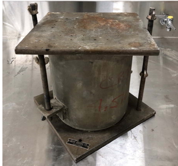
Figure 5: Modified CBR Test Assembly
