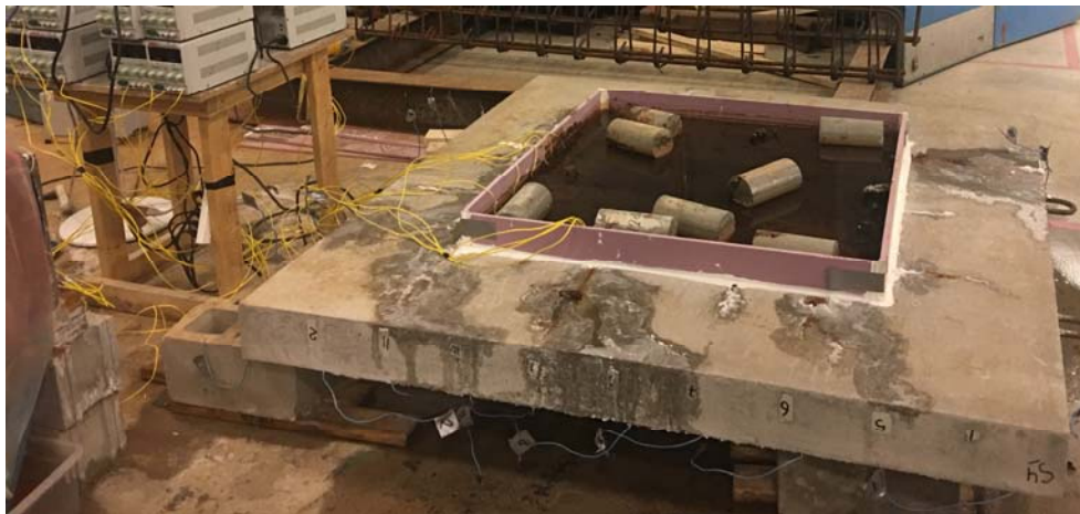
Figure 4: Constant current accelerated corrosion technique setup
