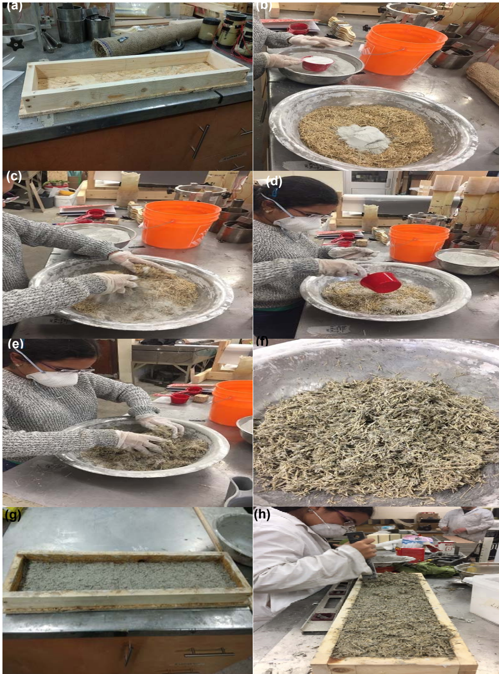
Figure 1: Specimen preparation: (a) formwork; (b) adding binder to flax; (c) mixing binder with flax; (d) adding water to mix; (e) mixing water with flax and binder; (f) finally obtained mix; (g) formwork filled to half to place burlap; and (h) casting and compaction
