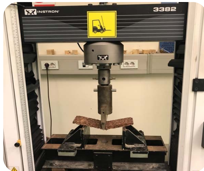
Figure 4: The Universal Testing Machine with the Sample
