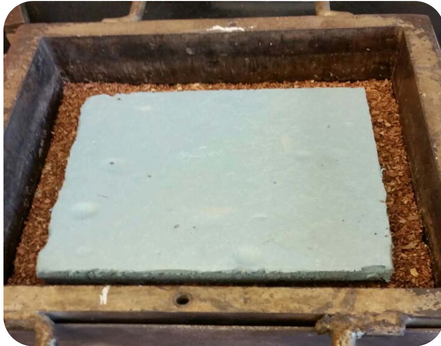
Figure 2: The Extruded Polystyrene after being placed above the lower layer of the panel.
