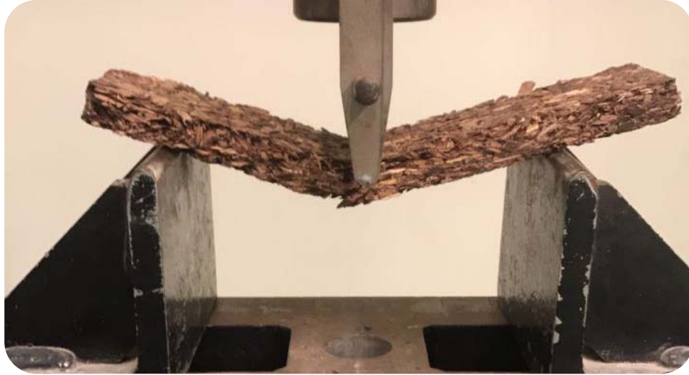
Figure 6: The specimen at point of failure.
