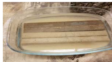
Figure 6: Mortar bar specimens
