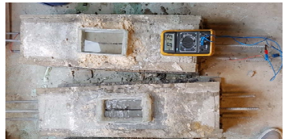
Figure 5: Corrosion beams with extruding reinforcement
