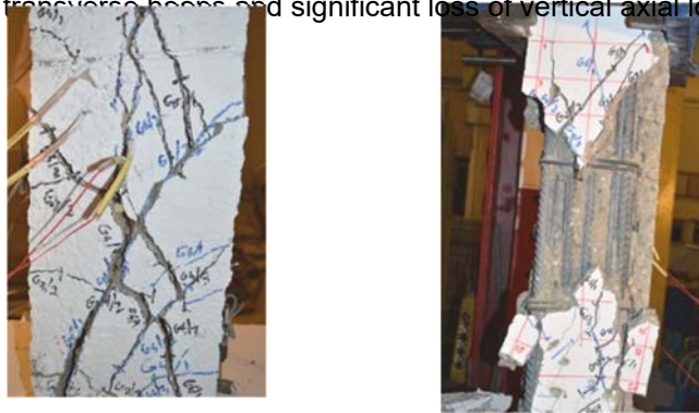
Figure 10: Failure mode of specimen S40
