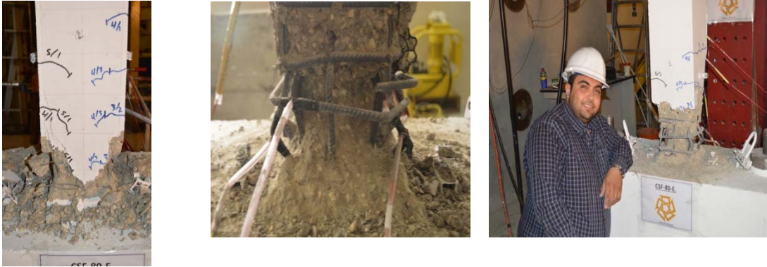
Figure 7: Failure mode of specimen F80
