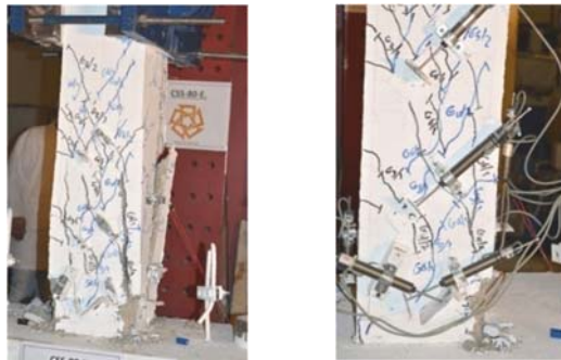
Figure 12: Initial and final failure mode of specimen S80
