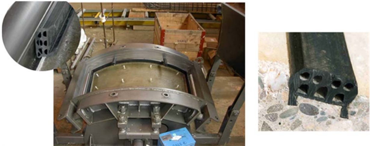
Figure 11: Anchored gaskets fixed into concrete segment during segment production without using glue.
