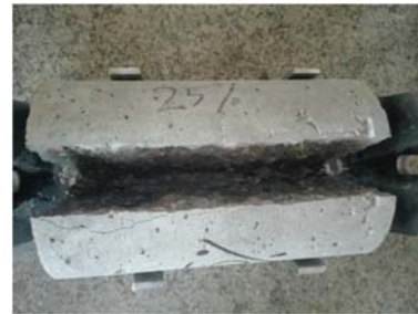
Figure 4: SCC sample after splitting
