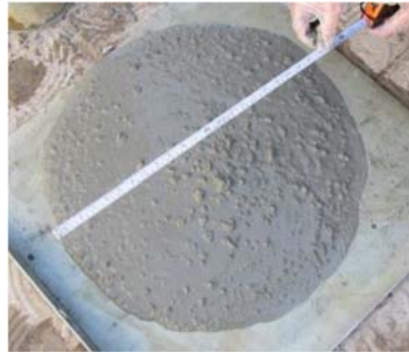
Figure 1: Slum flow test on SCC
