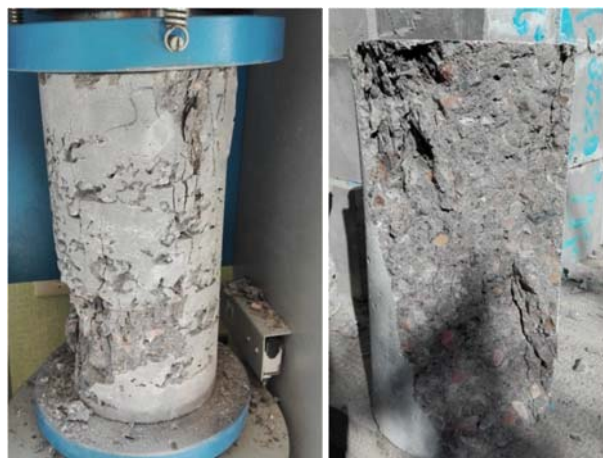
Figure 2: Rupture behavior of SCC caused by compressive strength test
