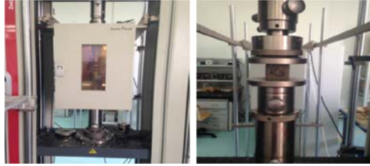
Figure 3 The equipment used for the compressive strength testing under room temperature and higher temperatures
