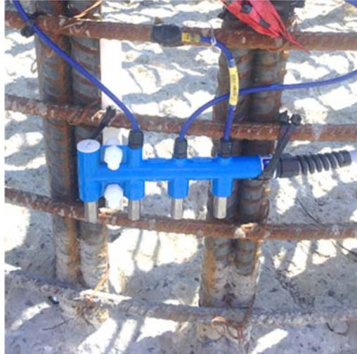
Figure 5: Corrosion sensor (embedded)
