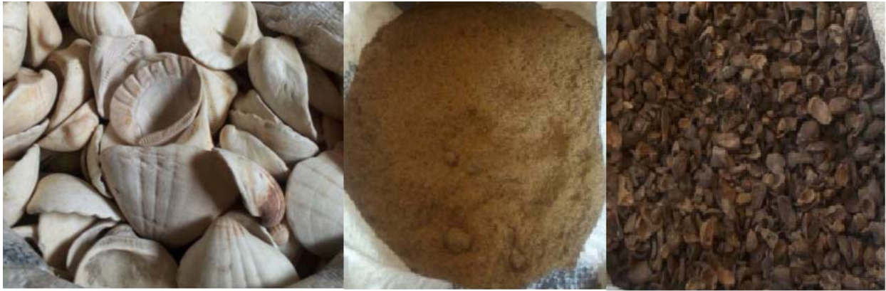
Figure 1: Clamshells, Rice Husk and Palm Oil Fuel Shells in their raw form
