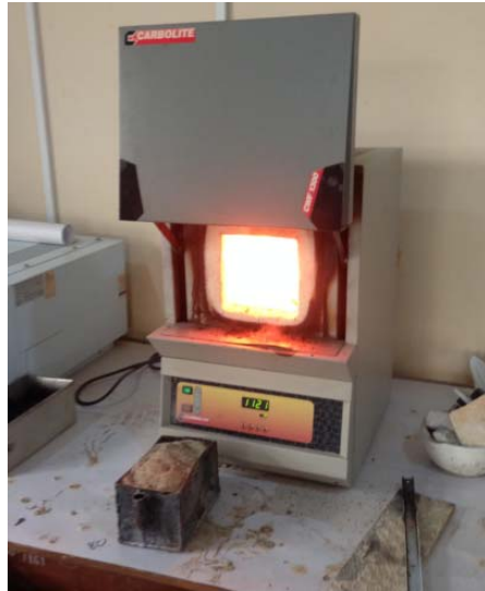
Figure 3: Incineration of materials inside the furnace
