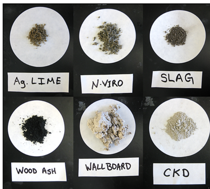
Figure 1: Gypsum wallboard residuals and additives used in this study
