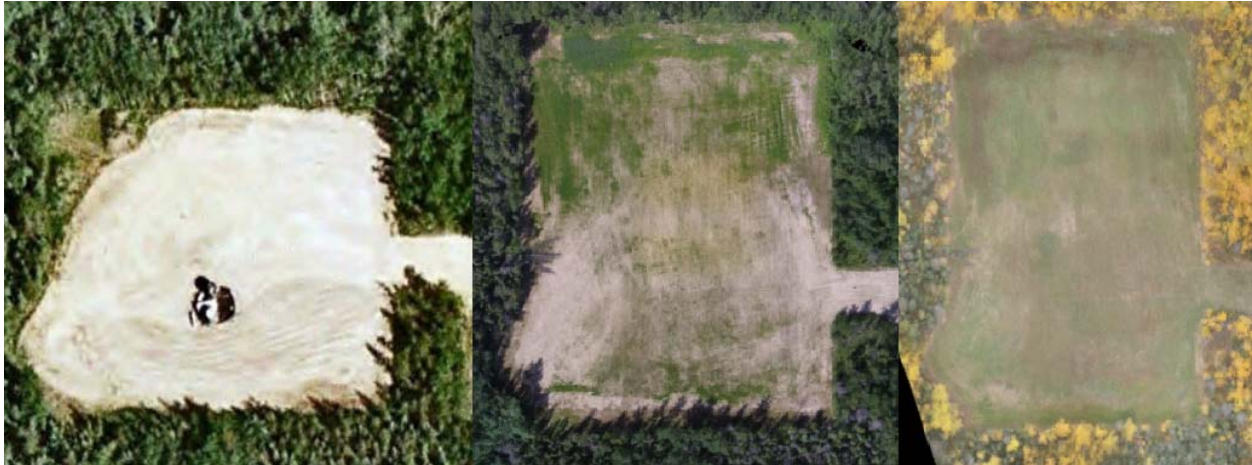
Figure 5: Restoration progress of well pad 4: 2012 (Google Earth), July 2017, and September 2017
