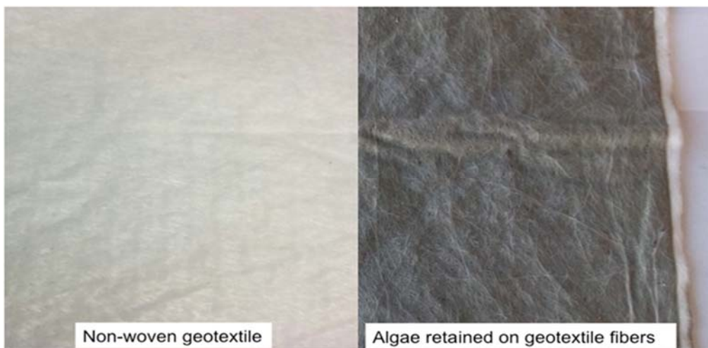
Figure 3. Non-woven geotextile before and after filtration
