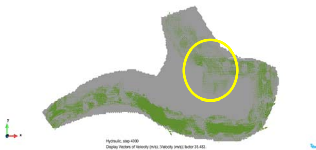
Fig 4e. Velocity vector field Q = 1306.2 \text{ m}^3/\text{s} .
