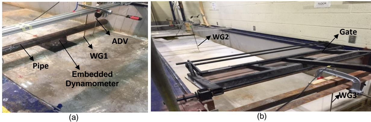
Figure 2: a) Side view, pipe, ADV and wave gauge, b) side view - flume and gate.
