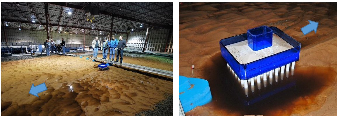
Figure 5. Comprehensive physical model of Port Mann showing scour at Pier N1 (NHC 2009a)
