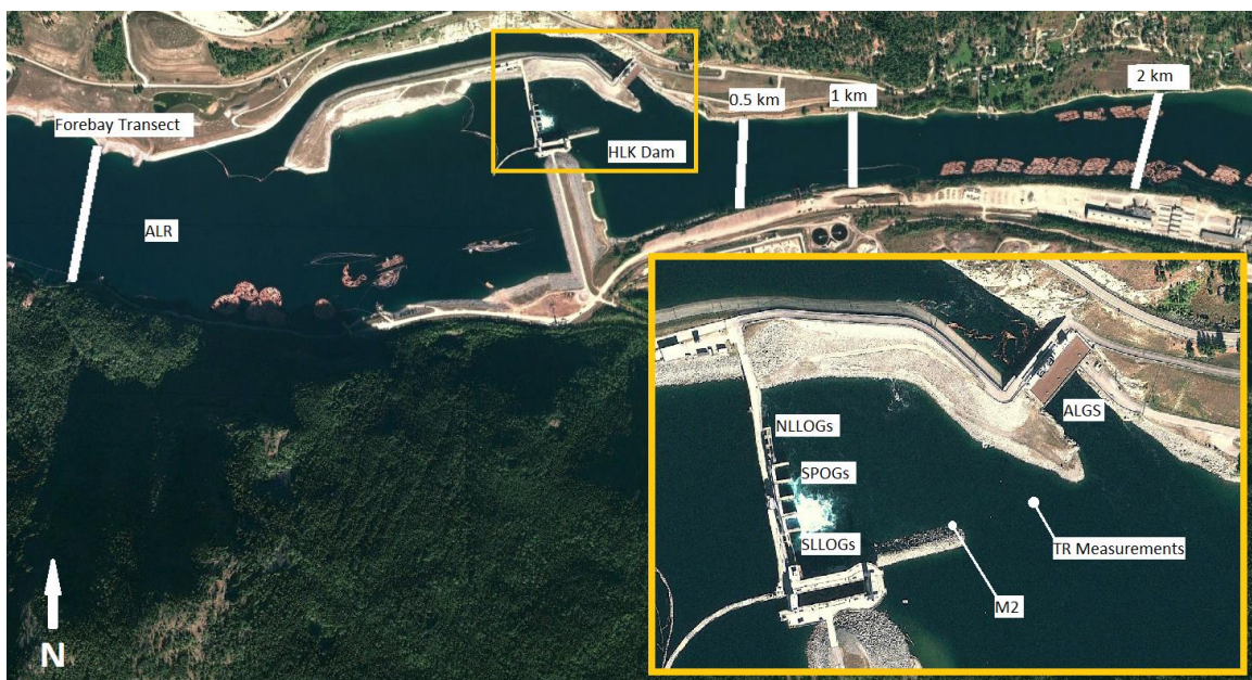
Figure 1: HLK dam site on the Columbia River and downstream river transects, tailrace (TR) measurement location, and Bruce (2016a) meter 2 (M2)
