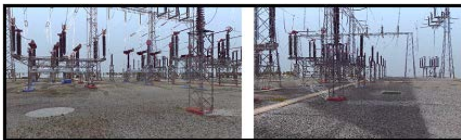
Figure 3: Sample of scanned point cloud of power facilities using PhotoModeler
