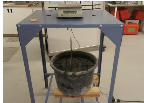
Figure 6: Measurement of the weight in water using a chain hooked to the weight balance.
