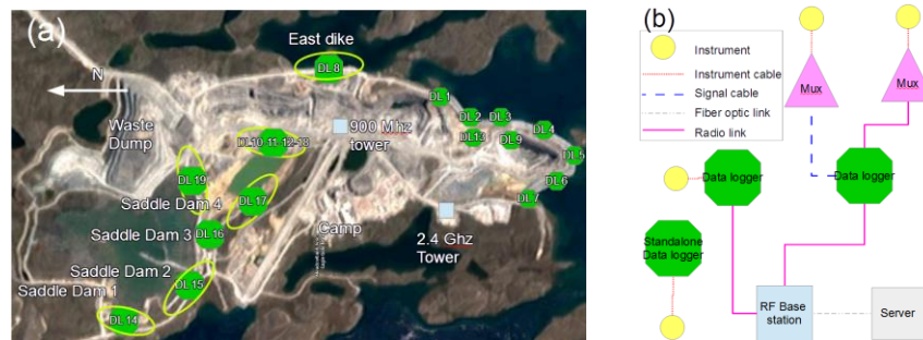
Figure 1 : (a) overhead view of the logger network (b) Schematics describing the standard setup of the system
