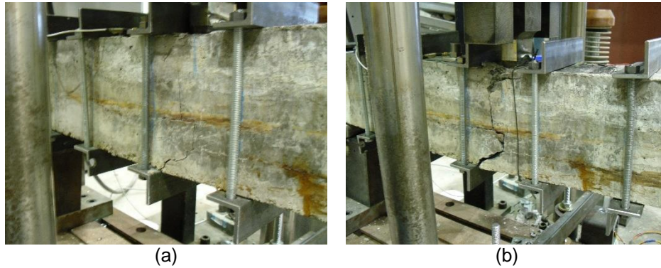
Figure 7: Post-test photos of Beam 2 (DOC 2.67%): (a) post 175-mm (b) post 200-mm
