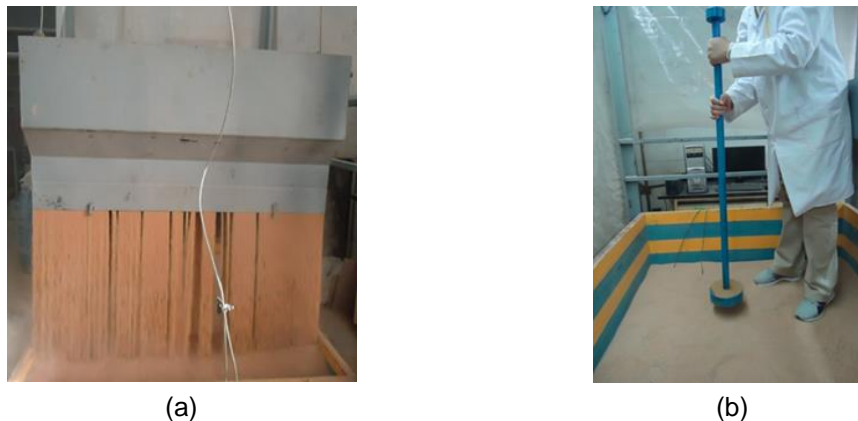
Figure 4: Preparation of sand layer. a) Sand raining technique b) Preparation of dense sand using tamping.
