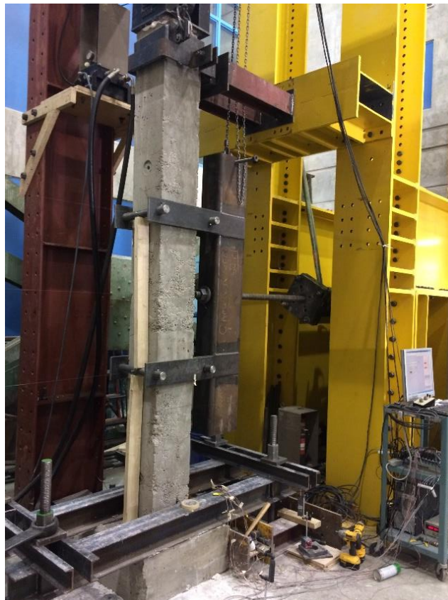
Figure 2: Photograph of experimental setup for residual capacity.
