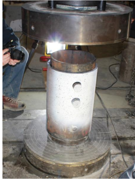
Figure 3: Specimen of mechanical connection before test.
