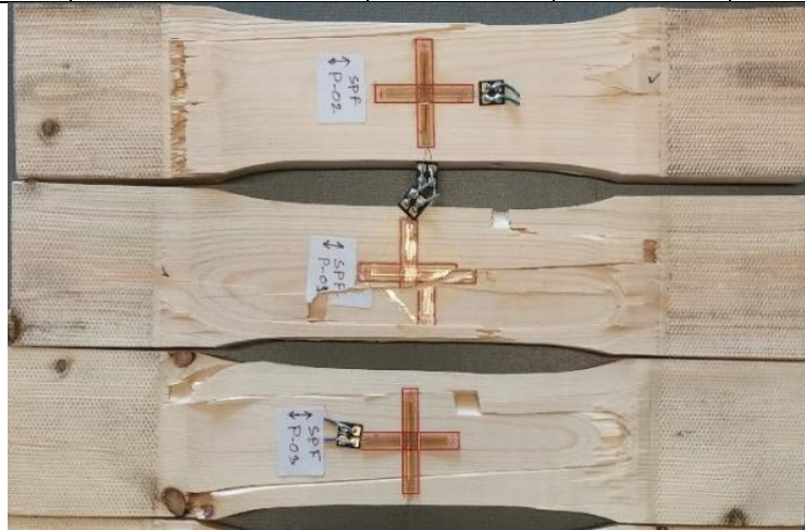
(a) Tested Timber Specimens (SPF) subjected to tension parallel to fiber
