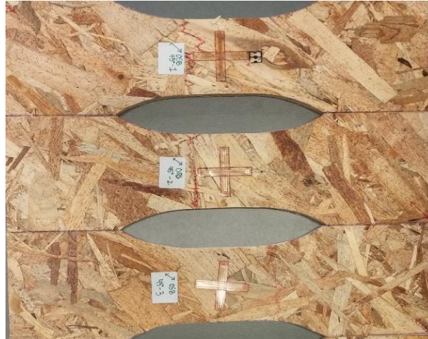
(a) Tested OSB Specimens (Diagonal ( D45^0 ) direction)
