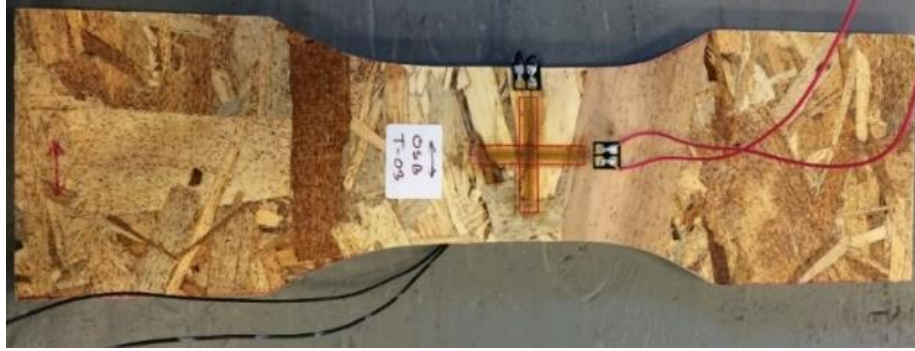
Figure 2 Sample of a OSB Tension test specimen with a Bi-axial Strain Gauge
