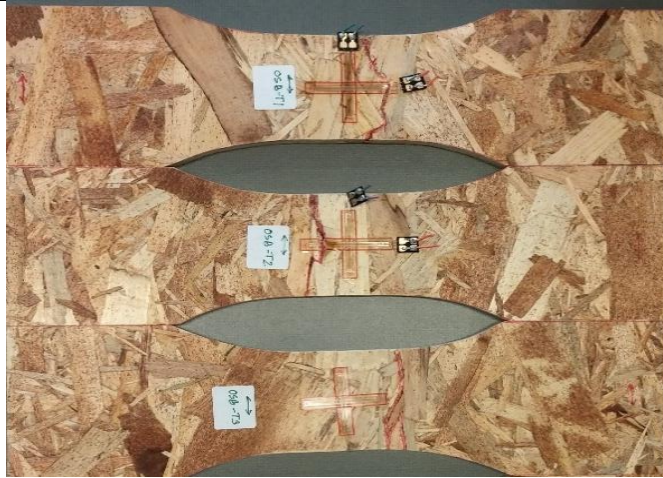
(a) Tested OSB Specimens (Transverse direction)
