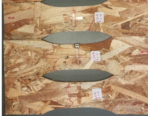
(a) Tested OSB Specimens along Strong Axis (Longitudinal direction)
