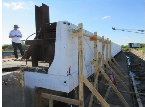
Figure 10: View of the loading setup and sensors' supporting frame at exterior location of the barrier
