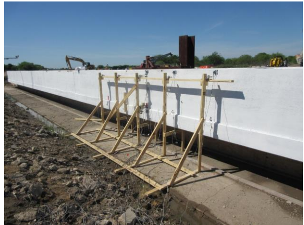
Figure 12: View of the timber frame supporting petontimeters at interior location
