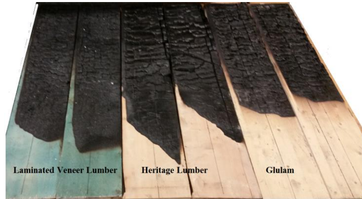
Figure 10. Timber Specimens after Heating.
