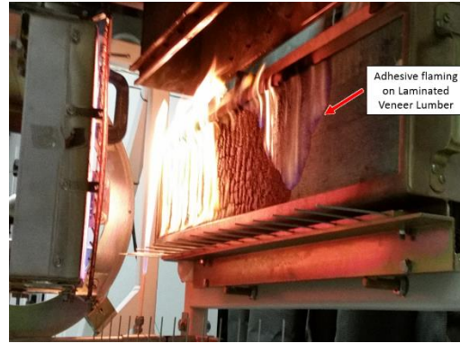
Figure 3. A contemporary flame spread test on laminated veneer lumber (LVL) conducted by the authors using a LIFT (Lateral Ignition and Flame spread Test) apparatus. In this test, adhesive flaming was observed demonstrating the complexity of modern engineered timber. The flame front of the adhesive would be quantified and a spread rating implied on the material (see Otto et al., 2017).
