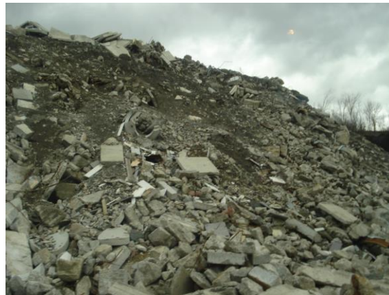
Figure 1: Construction and Demolition waste is a problem. Various quarries are now accepting this waste and marketing it as Recycled Concrete Aggregates as shown in this photo of a stockpile taken at a Quarry in Ottawa, Canada.
