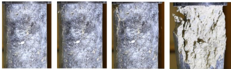
Figure 7: Failure progression time lapsed of 100% recycled cement substitution
