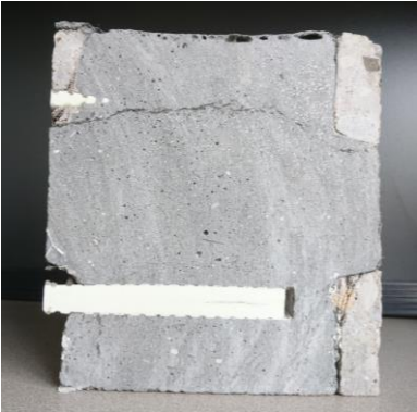
Figure 6: View of bar slippage in a sliced core sample
