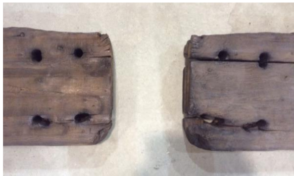
(a) Burned glulam beam sections with the char layer removed
