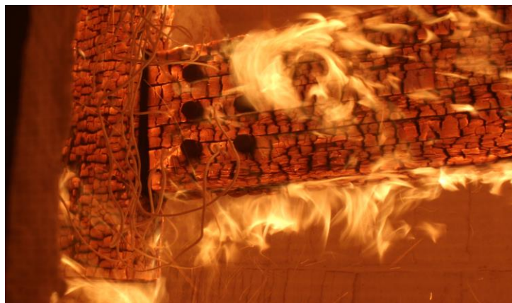
Figure 4: Beam-column test assembly with six bolts in three rows exposed to a standard fire.
