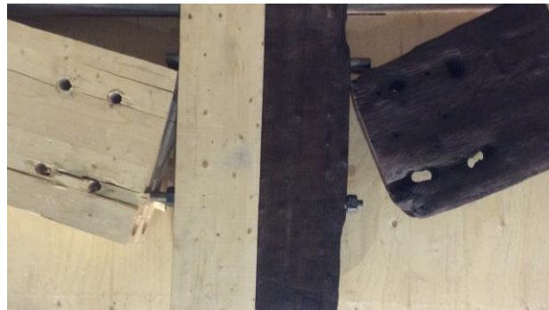
(b) Comparison between two similar connections with and without fire exposure
