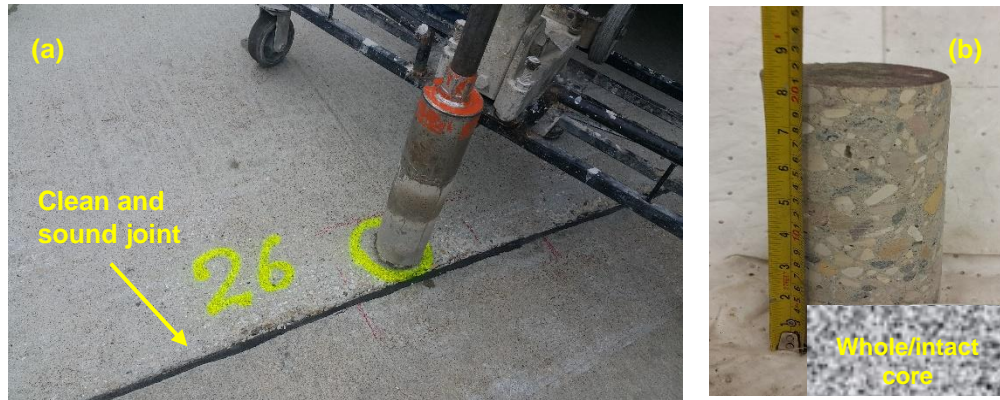
Figure 3: An example from a residential street showing: (a) sound joint without evidence of faulting or spalling, and (b) whole/intact core.
