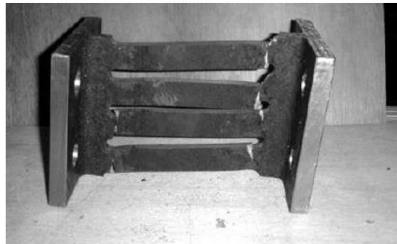
Figure 1: Damage at the strip ends due to stress concentration (adapted from Chan et al. 2008)
