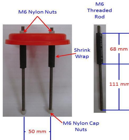
Figure 3: Electrodes setup for fresh cement paste electrical resistivity measurement (photo courtesy of Giatec Scientific Inc., 2015)
