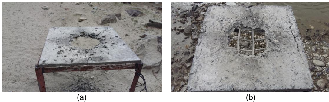
Figure 2: Preliminary tests for contact explosion on (a) PC slab (b) RC slab
