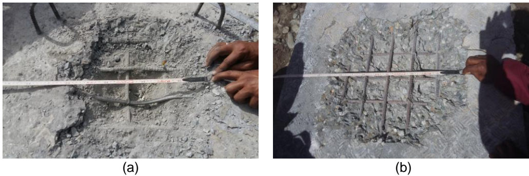
Figure 4: (a) Crater on detonated face (b) Scab diameter at bottom face
