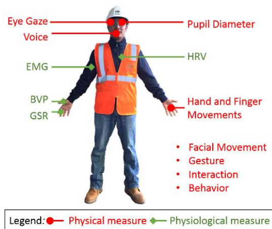
Figure 1: Common physical and physiological measures and their usual sources for the measures (adapted and modified from Sharma and Gedeon, 2012).
