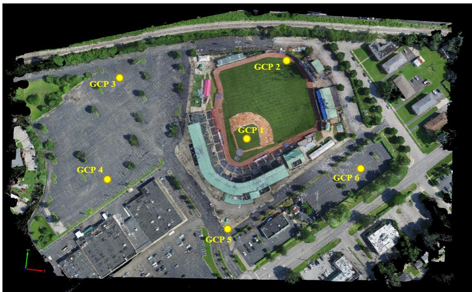
Figure 8: Distribution of GCPs in the 3D Point Cloud Model of the Stadium
