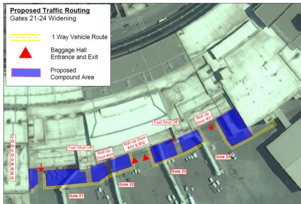
Figure 9: Exterior Site Layout
