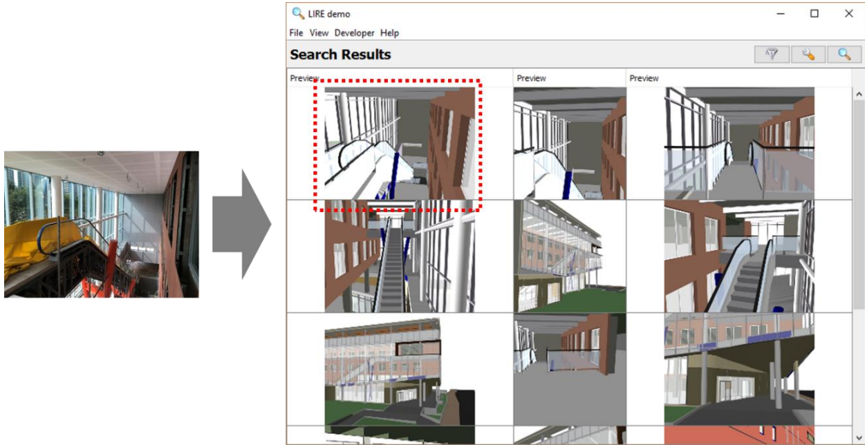
Figure 3: Example of the most similar image search process using LIRE (Case 1, EHD)
