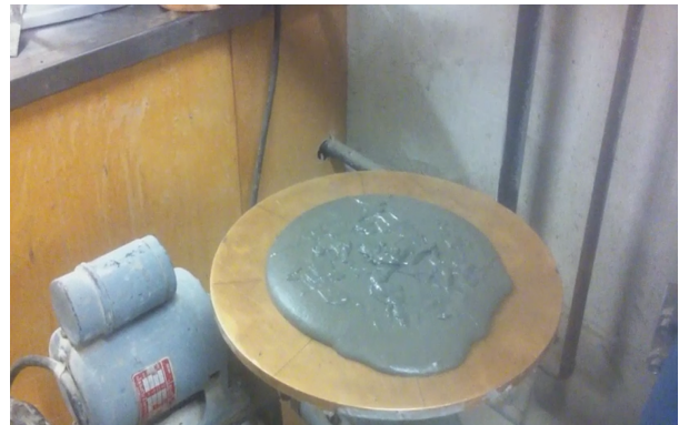
Figure 7. View of the 171 mm flow of XSFSLWR1-06 without fibers and without impacts
