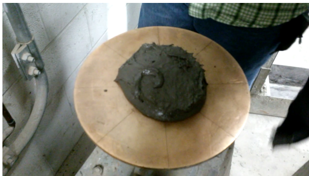
Figure 8. View of the 165 mm flow of XSFSLWR1-06-fib2% without impacts
