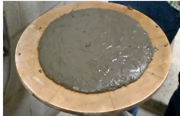
Figure 11. View of the 221 mm flow of XSFLWR5-06-fib2% without impacts
