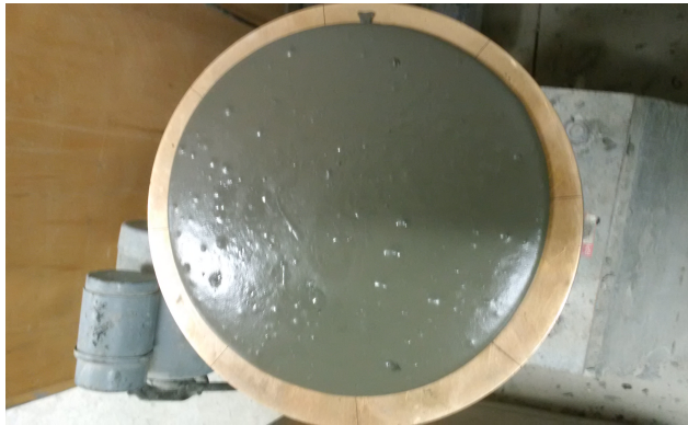
Figure 10. View of the 225 mm flow of XSFLWR5-06 without fibers and without impacts
