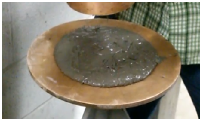
Figure 12. View of the 180 mm flow of mix XSFLWR5-06-fib2% without impacts and after 25 minutes from mixing
