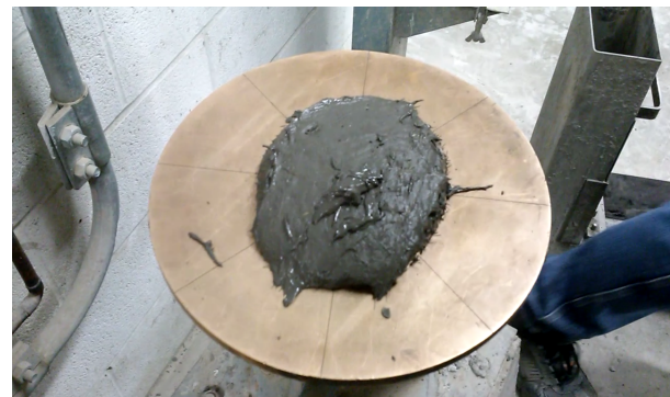
Figure 9. View of the 154mm flow of XSFSLWR1-06-fib1.5% without impacts
