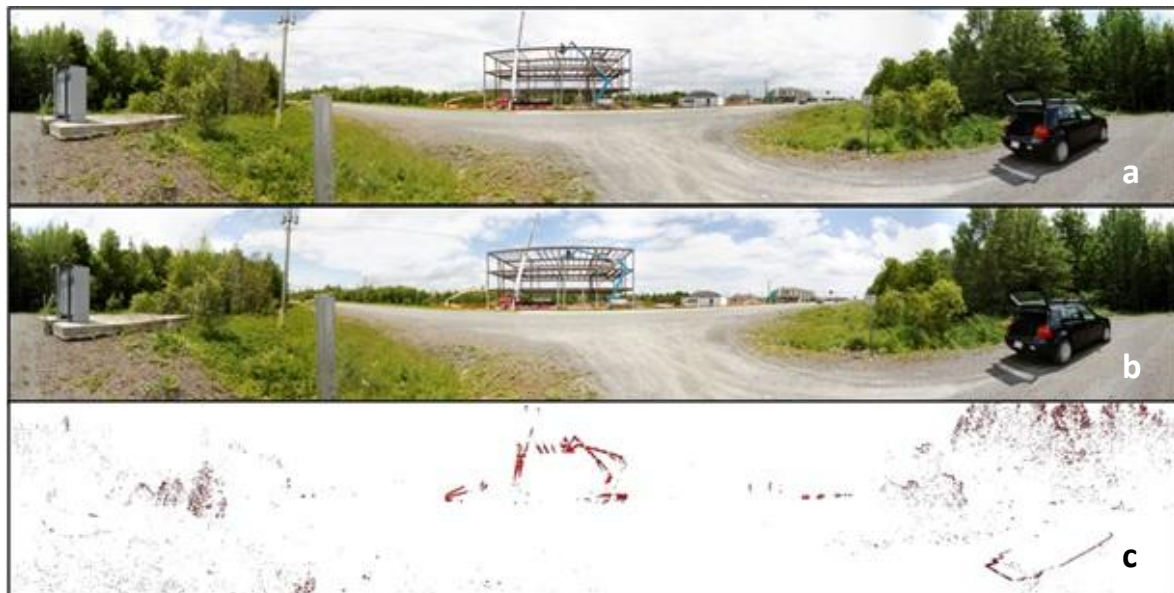
Figure 7: On-site testing: (a) Base state, (b) Objects moved, (c) Final change mask
