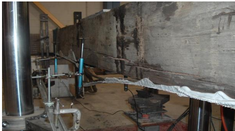
Figure 10: De-bonding of the Hardwire Sheet in the Tension Zone
