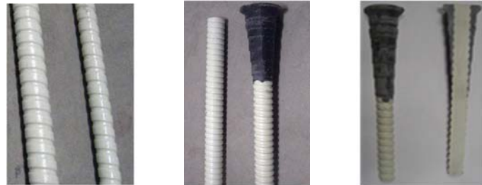
(a) Bar shape (b) Headed-end bar (c) Sliced head Fig. 4 Configurations of the used GFRP bars
