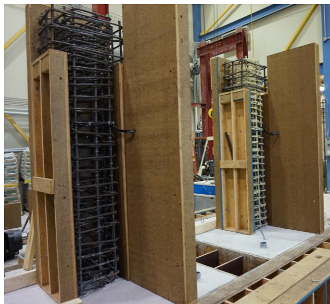
Figure 2: Construction process for the test specimens
