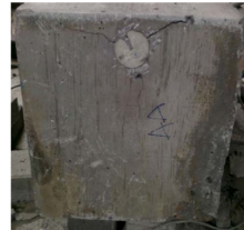
(b) Bar slippage from the anchorage head and V-shape side concrete cover crack in case of embedment length of 76 mm with bar head in case of #6 GFRP Bar (BS-VSCCC)
