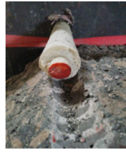
(a) Bar head breakage followed by bar slippage and concrete splitting (HB-BS-CS)
