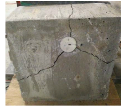
(a) Bar slippage from the anchorage head followed by concrete splitting (BS-CS)
