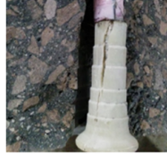
(a) Bar head breakage followed by bar slippage and concrete splitting (HB-BS-CS)
