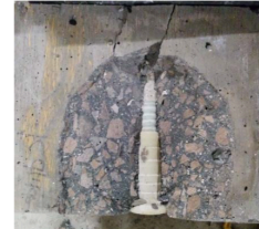
(b) Bar slippage from the anchorage head and V-shape side concrete cover crack in case of embedment length of 76 mm with bar head in case of #6 GFRP Bar (BS-VSCCC)
