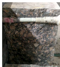
(a) Bar slippage from the anchorage head followed by concrete splitting (BS-CS)
