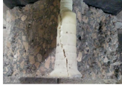
(a) Bar head breakage followed by bar slippage and concrete splitting (HB-BS-CS)
