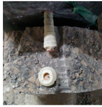
(a) Bar head breakage followed by bar slippage and concrete splitting (HB-BS-CS)
