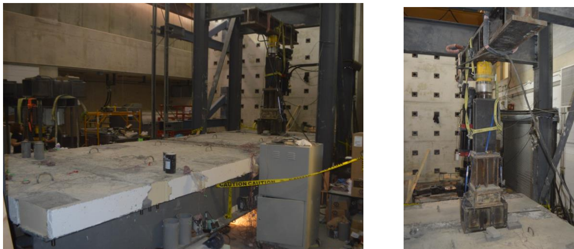
a. Slab-girder bridge system during monotonic loading b. View of loaded area Figure 5. View of the test setup for the monotonic loading
