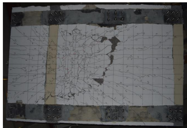
a. Top view of the slab showing punching shear failure at the footprint of the wheel load b. Bottom view of the slab showing crack pattern after failure
