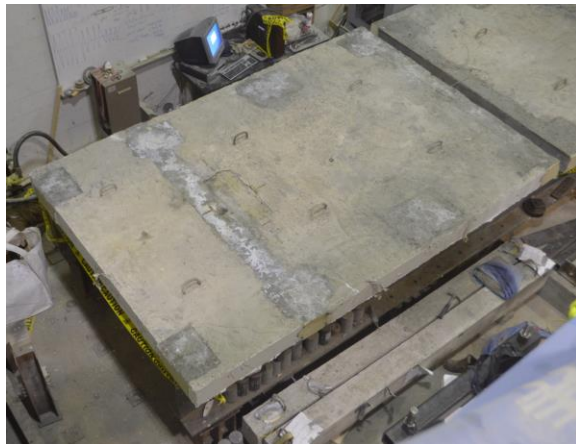
a. Top view of the slab showing punching shear failure at the footprint of the wheel load b. Bottom view of the slab showing crack pattern after failure
