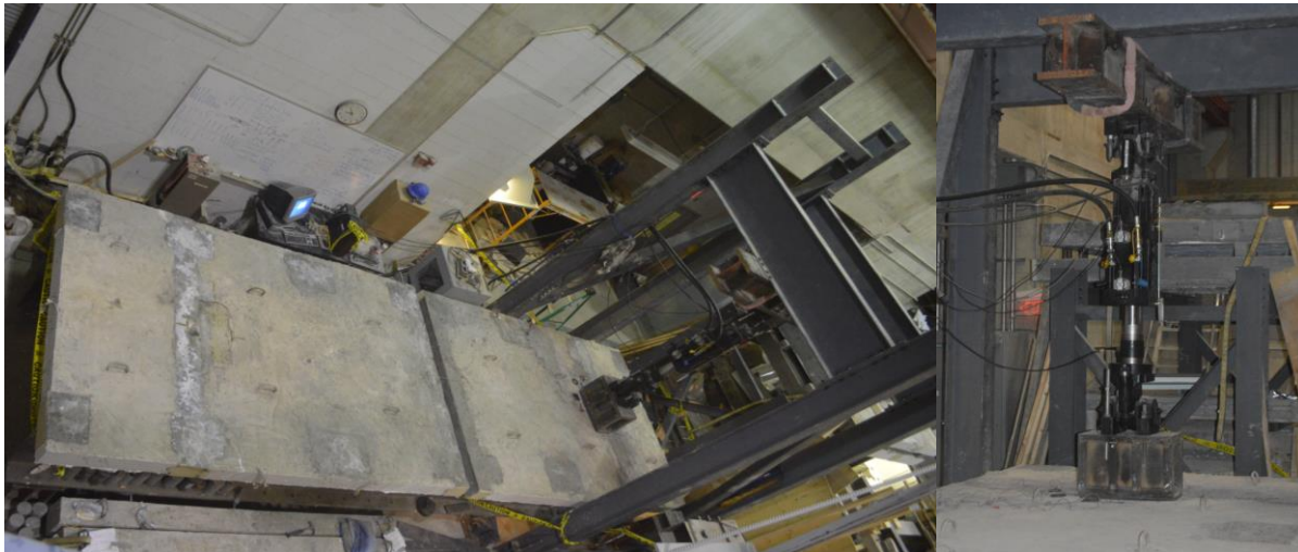
a. Slab-girder bridge system during CAF and VAF loading b. close-up view for the actuator Figure 4. View of the test setup for fatigue loading
