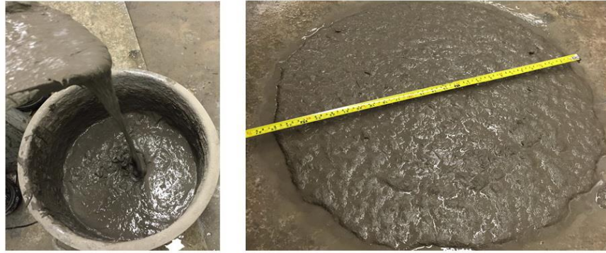
Figure 2: Best mixing procedure for ECC mixtures incorporating SAP particles.
