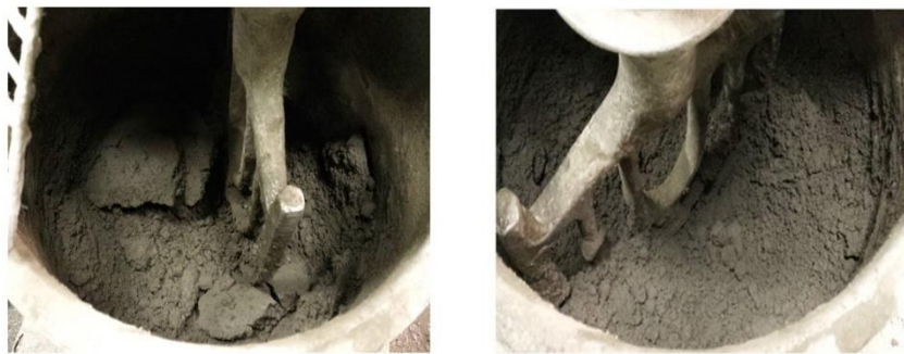
Figure 4: Harsh mix with low moistened after adding SAP particles.
