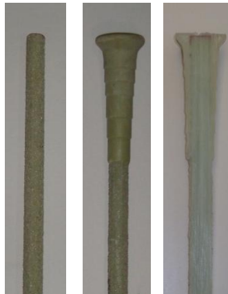
Fig. 2 Views of GFRP bars
