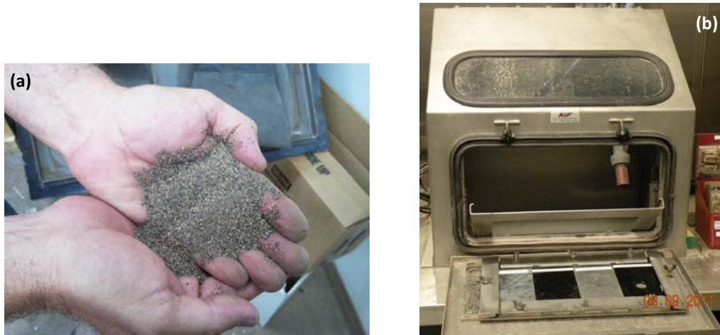
Figure 1: Abrasion testing was completed following internal procedures defined by MTQ using Ottawa silica sand (a) and a controlled abrasion test apparatus (b).
